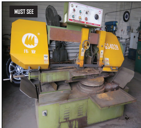
ZHEjiang Weiye / GY mdl. GS4028 12" Horizontal Band Saw s/n 12103006 w/ Manual Clamping, Coolant
