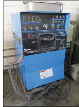
Miller Syncrowave 350LX CC-AC/DC Squarewave Welding Power Source w/ Bernard Cooler.
