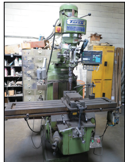
2012 Takam TK-4 Vertical Mill s/n 208055 w/ Rational WE6800-2 Programmable DRO, 3Hp, 80-5440 RPM, 16-Speeds, Chrome Box Ways, Power Feed, 10" x 50" Table.
