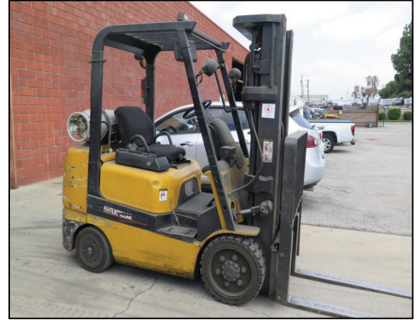
Caterpillar GC25K-HP 4700 Lb Cap LPG Forklift s/n AT820-90448 w/ 3-Stage Mast, 188" Lift Height, Side Sift, Solid Tires, 10,220 Hours.
