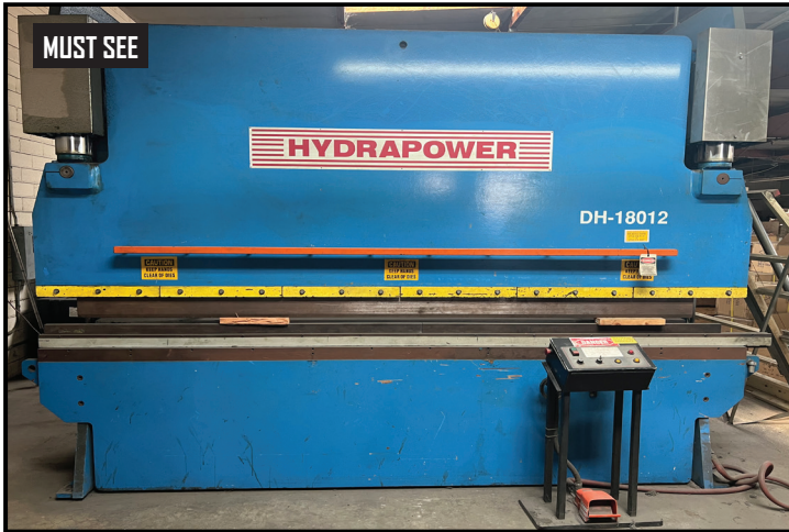
Hydrapower DH-18012 180 Ton x 12' Hydraulic Press Brake s/n T3087 w/ Manual Back Gauge, 12' Bed Length, 8 3/4" Throat.
