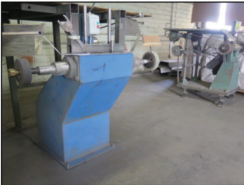
7.5Hp Polishing Mill (Buffer) w/ 30" Throat.
