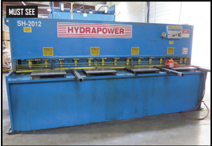
Hydrapower SH-2012 12' x 1/4" Hydraulic Power Shear s/n 03086 w/ Dial Back Gauge, 99" Squaring Arm, Front Supports.
