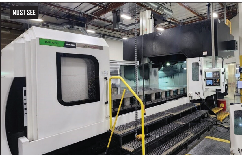
HMG) 2018 HMG HAS-423EAY Double Column Bridge Type Machining Center, 10,000 RPM, 157.48" x 122.03" x 39.37" (XYZ), 32 ATC, BT 50, Table Size 157.48" x 86.61", Spindle Nose to Table Top (13.78" -53.15"), Fanuc OIMF Control, Chip Conveyor, (Moved to Livermore, CA from Fremont, CA for Convenience of Sale)
