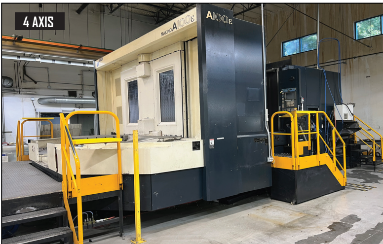
2003 Makino A100E CNC Horizontal Machining Center, 1000 mm Dual Pallet, 39.4" x 39.4" Pallet Size, 66" x 53" x 55" (XYZ), 132 ATC, 12,000 RPM, CAT 50, Makino Professional 3 CNC Control, Full 4th Axis, 40 HP, Chip Conveyor, 1000 PSI High-Pressure Coolant.
