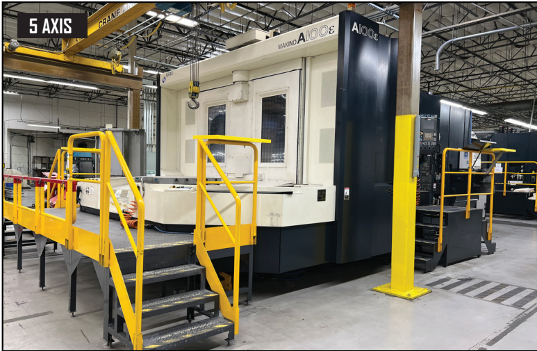
2006 Makino A100E-5XR CNC Horizontal Machining Center, 1000 mm Dual Pallet, 39.4" x 39.4" Pallet Size, 66" x 53" x 55" (XYZ), 132 ATC, 18,000 RPM, CAT 50, Makino Professional 5 CNC Control, Full 4th Axis, 40 HP, Chip Conveyor, 1000 PSI High Pressure Coolant.
