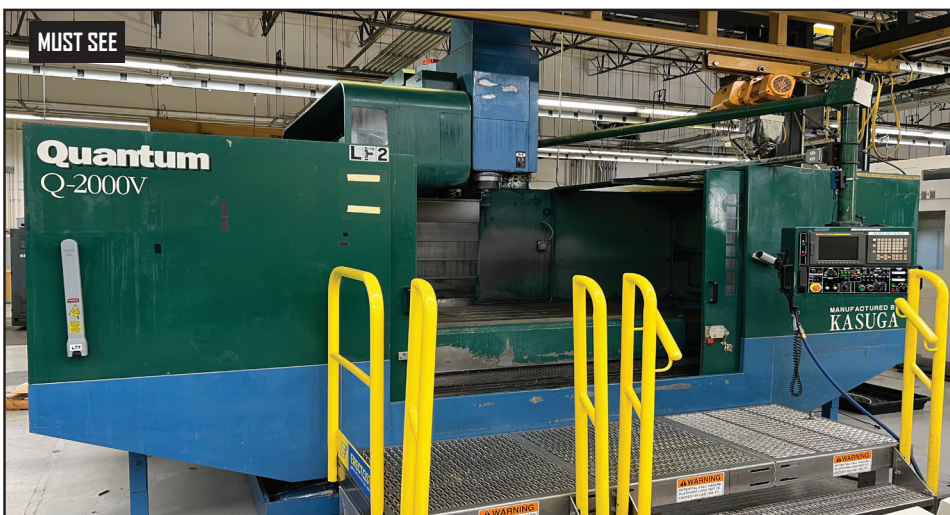
Kasuga Quantum Q-2000V CNC VMC, 50 Taper, 80" x 30" x 20" (XYZ), 30 ATC, Fanuc 18I-M Control, Dual Chip Conveyor, 6000 RPM, 3 Axis.
