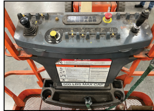
2006 JLG MODEL E400AN ARTICULATING BOOM LIFT, 500 LB CAPACITY, 48V, 40FT MAX PLATFORM HEIGHT, 21.2 FT MAX HORIZONTAL REACH.
