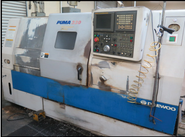
2001 Daewoo PUMA 2300 CNC Turning Center w/ Fanuc 21i-T Controls, Tool Presetter, 10-Station Turret
