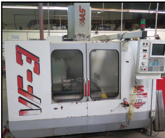
1997 Haas VF-3 4-Axis CNC VMC w/ Haas Controls, 20-ATC, CAT-40 Spindle, 7500 RPM, Rigid Tapping
