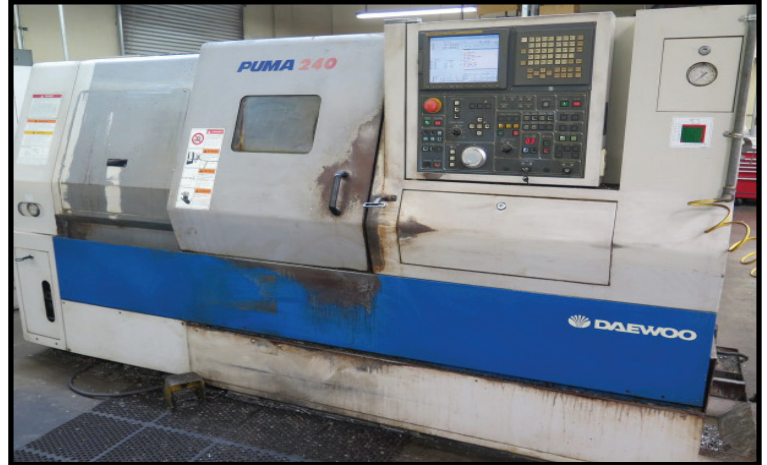
2004 Daewoo PUMA 240B CNC Turning Center w/ Fanuc 21i-TB Controls, Tool Presetter, 12-Station Turret
