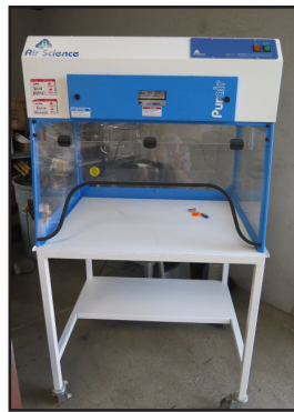
Air Science Purair mdl. P5-36 Ductless Flow Hood
