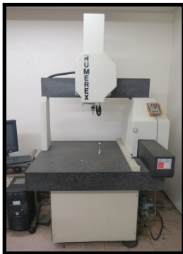
Numerex 2428-18 CMM Machine w/ Renishaw PH1 Probe Head, 24" x 28" x 18" Work Envelope 3954 J & L 14" Optical Comparator w/ Acu-Rite DRO, Surface and Profile
