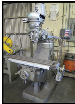
Sharp YC-1 1/2 VA Vertical Mill w/ Anilam Mini Wizard DRO, 1.5Hp Motor, 80-2720 RPM
