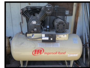
Ingersoll Rand 2545E10V2 10Hp Horizontal Air Compressor w/ 2-Stage Pump, 120 Gallon Tank
