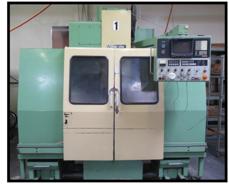
Mori Seiki MV-40B CNC Vertical Machining Center w/ Fanuc 10M Controls, 20-Station ATC, CAT-40 Taper Spindle, 17 3/4" x 43" Table
