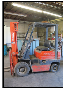
Toyota 40-5FG15 3000 Lb Cap LPG Forklift w/ 2-Stage Mast, Yard Tires
