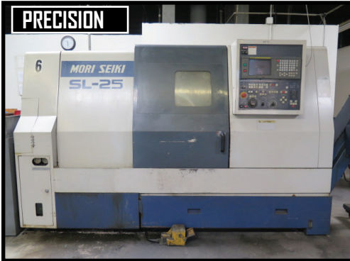
Mori Seiki SL-25B5 CNC Turning Center w/ Fanuc MF-T6 Controls, Tool Presetter, 12-Station Turret, Hydraulic Tailstock, 10" 3-Jaw Power Chuck, Chip Conveyor
