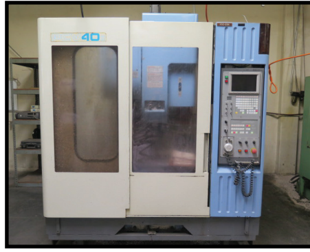
OKK PCV40 II-HS CNC Vertical Machining Center w/ OKK Neomatic Controls, 20-Station ATC, CAT-40 Taper Spindle, 16" x 28 1/4" Table
