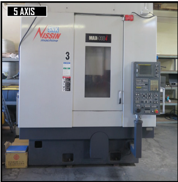
2007 SNK Nissen MAX-410i 5-Axis CNC Vertical Machining Center w/ Fanuc Series 18i-MB Controls, 28-Station ATC, CAT-40 Taper Spindle, Trunnion Style 16 3/4" Rotary 4 th /5 th Axes, Chip Auger, Chip Conveyor
